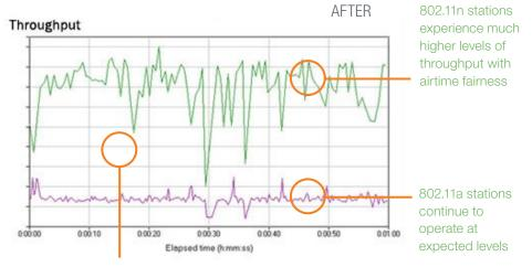
Transmit queues scheduled based on the airtime constraints per station using weighted round robin algorithm
